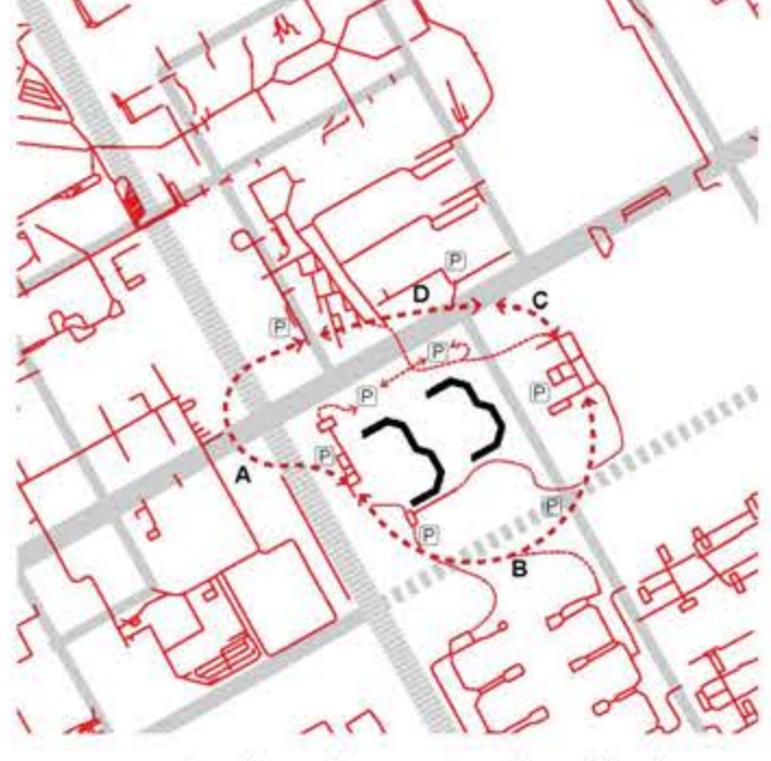
we propose to phase the construction of the loop, before starting work on the dreven; the loop builds on the existing infrastructure.
